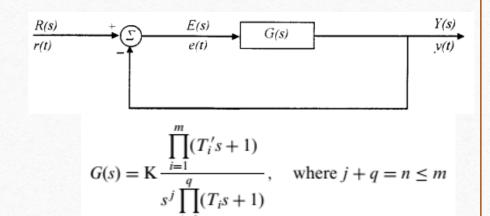
Consider the closed- loop system of unity feedback of Figure. The system error e(t) is defined as the difference between the command signal r(t) and the output of the system y(t).
