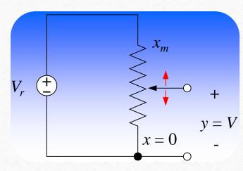
A linear potentiometer used as position sensor is a zero-order sensor.
